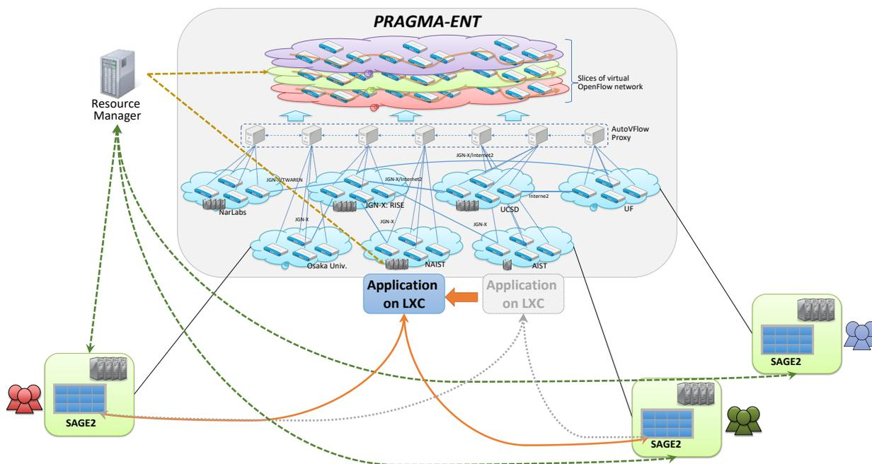
Figure 2 System structure of Software-Defined IT infrastructure
