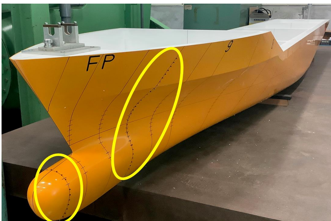
Fig. 3 Turbulent stimulator on the bow of the model ship
