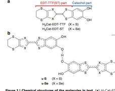
Figure 1 Chemical structures of the molecules in text. (a) H<sub>3</sub>(Cat-EDT-TTF) and H<sub>3</sub>(Cat-EDT-TTF-D). (b) A hydrogen-bonded molecular unit, x-S and x-Se.
