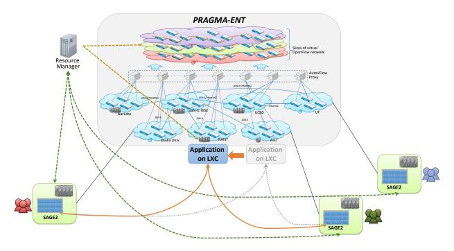
Figure 2 System structure of Software-Defined IT infrastructure
